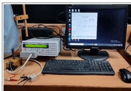
Fig 1: LCR meter setup for dielectric measurement.
