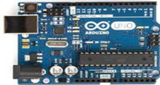
Fig-2: Arduino UNO R3 development card
