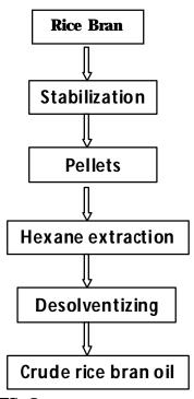
FIG. 2: Process for rice oil production.
