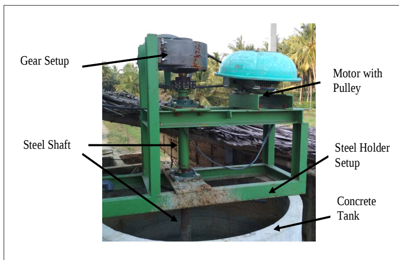
Fig 2: Block representation of mixer setup (Cowdung, urine, jaggery, soil and gram flour).
