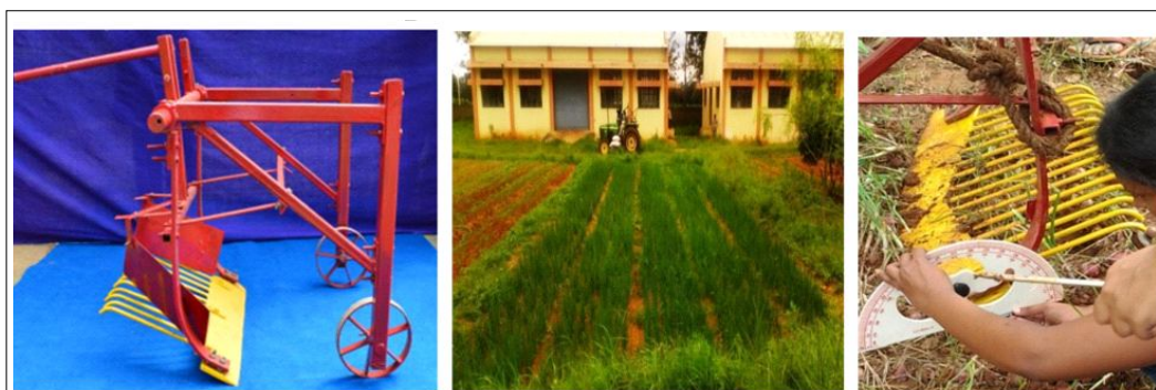
Fig 2: (A) Animal-drawn onion digger (B) Experimental plot with two onion varieties and (C) Rake angle adjustment to the digger during harvesting.
