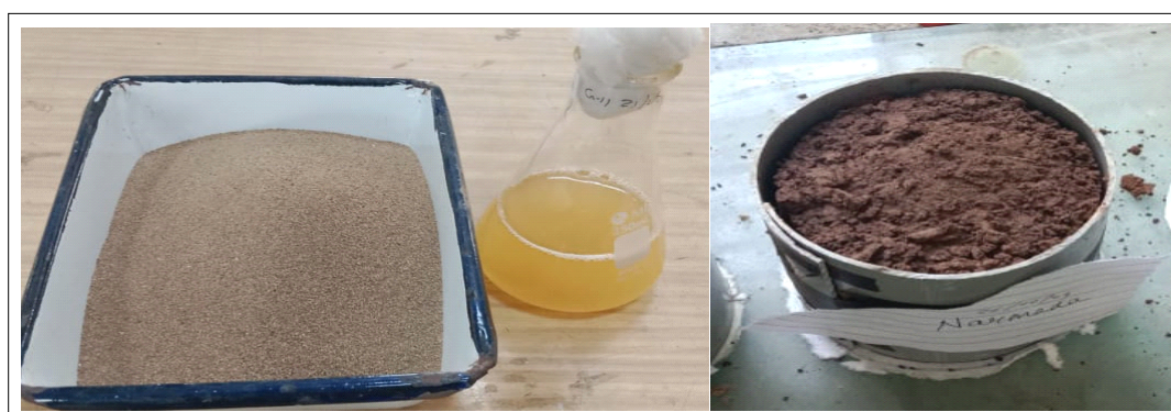
Fig 4: Preparation of mould: (1) Narmada soil sample with bacterial solution.
