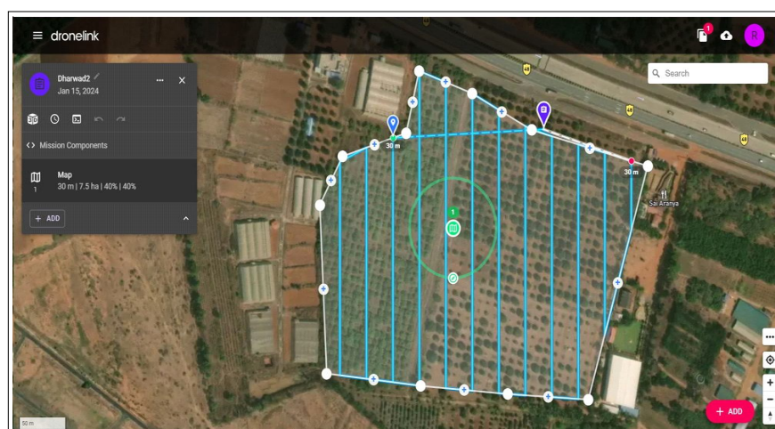
Fig 2: Drone navigation pattern view of the selection area in the dronelink application.
