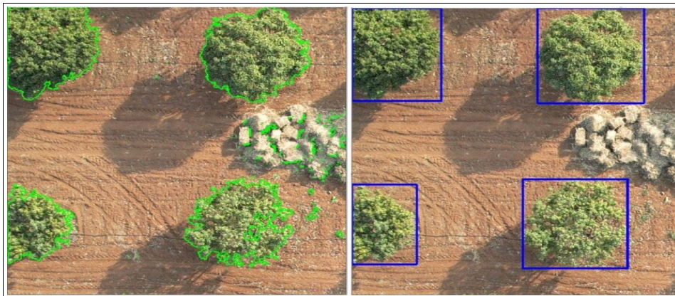
Fig 7: (a) Detected counters over the original image and (b) Bounding box drawn on the object with the area above threshold value.
