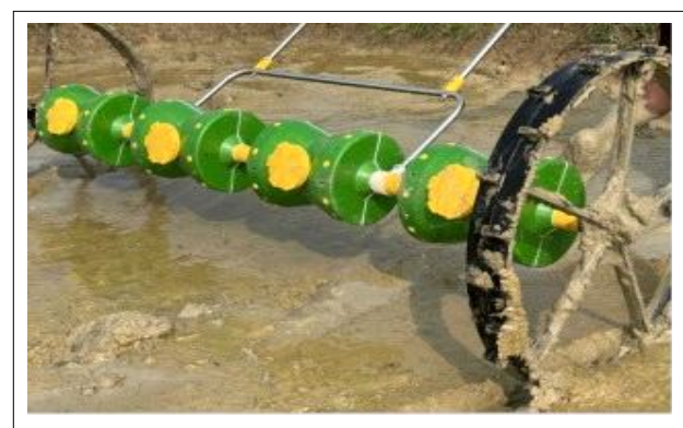
Fig 2: Dispense the sprouted paddy seeds evenly in the puddled field at the line spacing of 20 cm.
