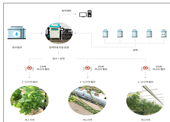
Fig 1: Smart farm nutrient solution system.
