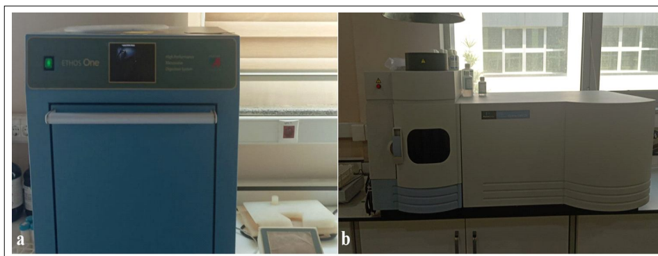
Fig 2: Analytical instruments (a. Milestone Ethos One digestion system, b. Perkin Elmer Optima 5300DV).
