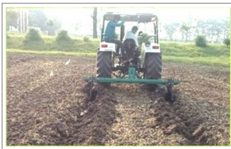
Fig 4: Tractor operated trencher for grape orchard.
